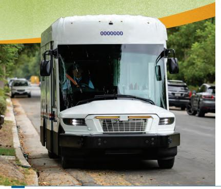
These BEVs, as they are known, are well suited to the Postal Service's mission. They are very effective at frequent stop-and-go driving, and the powertrain provides an immense amount of power to the vehicle, a real bonus when carrying heavy loads. BEVs also have fewer moving parts and use fewer fluids than vehicles powered by internal combustion, so there is less wear and tear and lower maintenance costs.
